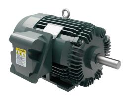
Toshiba SD premium efficiency AC induction motor, high-performance inverter duty and severe duty, 15hp, 3-phase, 230/460 VAC, 1200rpm, TEFC, NEMA 284T frame, cast iron, rigid base mount.
