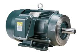
Toshiba SD premium efficiency AC induction motor, highperformance inverter duty and severe duty, 15hp, 3-phase, 230/460 VAC, 1800rpm, TEFC, NEMA 254TC frame, cast iron, Cface/rigid base mount.
