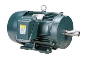
Toshiba SD premium efficiency AC induction motor, high-performance inverter duty and severe duty, 15hp, 3-phase, 230/460 VAC, 1800rpm, TEFC, NEMA 254T frame, cast iron, rigid base mount.
