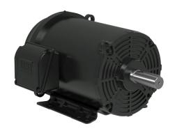
WEG Electric S premium efficiency AC induction motor, general purpose and inverter rated, 15hp, 3-phase, 208-230/460 VAC, 3600rpm, TEFC, 254T frame, rolled steel, rigid base mount.
