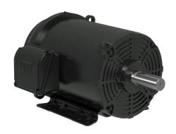
WEG Electric S premium efficiency AC induction motor, general purpose and inverter rated, 15hp, 3-phase, 208-230/460 VAC, 3600rpm, TEFC, NEMA 254T frame, rolled steel, rigid base mount.
