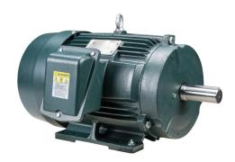
Toshiba SD premium efficiency AC induction motor, high-performance inverter duty and severe duty, 15hp, 3-phase, 230/460 VAC, 3600rpm, TEFC, NEMA 254T frame, cast iron, rigid base mount.
