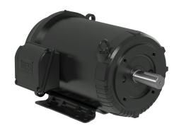
WEG Electric S premium efficiency AC induction motor, general purpose and inverter rated, 15hp, 3-phase, 208-230/460 VAC, 1800rpm, TEFC, NEMA 254TC frame, rolled steel, C-face/rigid base mount.
