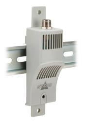
Stego Smart Sensor temperature/humidity sensor, -40 to 140 deg F, 0 to 100% RH, 4-20 mA output, 35mm DIN rail or panel mount, 4-pin M12 quick-disconnect.
