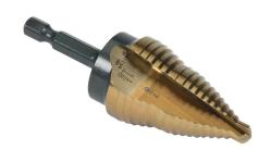
Viking step drill bit, 1/4in to 1-1/8in, size 1/4A, 16 steps, split point, high-speed steel (HSS), gold oxide finish, 1/4in hex shank, 3.0in (76mm) overall length.
