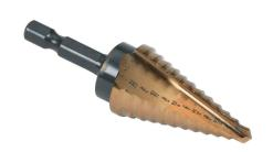
Viking step drill bit, 3/16in to 7/8in, size #8, 12 steps, split point, high-speed steel (HSS), gold oxide finish, 1/4in hex shank, 2.8in (71mm) overall length.
