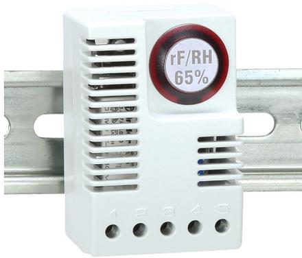
Stego electronic hygrosat, fixed, 65% relative humidity, 5% RH switching differential, 120 VAC operating voltage, 35mm DIN rail mount, for electrical enclosure climate control.
