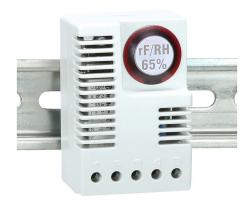
Stego electronic hygrostat, fixed, 65% relative humidity, 5% RH switching differential, 120 VAC operating voltage, 35mm DIN rail mount, for electrical enclosure climate control.
