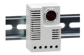
Stego electronic hygrostat, adjustable, 40% to 90% relative humidity, 5% RH switching differential, 120 VAC operating voltage, 35mm DIN rail mount, for electrical enclosure climate control.
