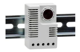
Stego electronic hygrostat, adjustable, 40% to 90% relative humidity, 5% RH switching differential, 230 VAC operating voltage, 35mm DIN rail mount, for electrical enclosure climate control.
