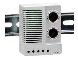
Stego electronic hygrotherm, adjustable, 32 to 140 deg F, 50% to 90% relative humidity, 3.6 deg F/4% RH switching differential, 100-240 VAC operating voltage, 35mm DIN rail mount, for electrical enclosure climate control.
