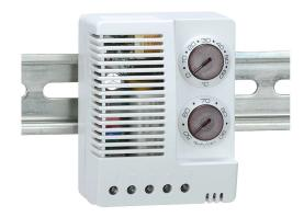
Stego electronic hygrotherm, adjustable, 0 to 60 deg C, 50% to 90% relative humidity, 2K/4% RH switching differential, 100-240 VAC operating voltage, 35mm DIN rail mount, for electrical enclosure climate control.
