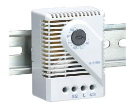
Stego mechanical hygrostat, adjustable, 35% to 95% relative humidity, 4% RH switching differential, 35mm DIN rail mount, for electrical enclosure climate control.
