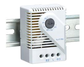
Stego mechanical hygrostat, adjustable, 35% to 95% relative humidity, 4% RH switching differential, 35mm DIN rail mount, for electrical enclosure climate control.
