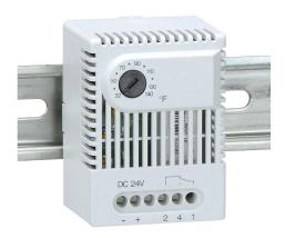
Stego electronic thermostat, adjustable, 32 to 140 deg F, 5.4 deg F switching differential, 24 VDC operating voltage, 35mm DIN rail mount, for electrical enclosure climate control.
