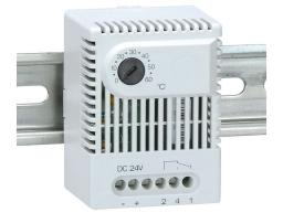
Stego electronic thermostat, adjustable, 0 to 60 deg C, 3K switching differential, 24 VDC operating voltage, 35mm DIN rail mount, for electrical enclosure climate control.
