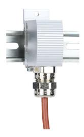
Stego thermostat, hazardous location rated, fixed, N.C. (open on rise) 59 deg F (15 deg C) switch-off, 9 deg F (5K) switching differential, 35mm DIN rail or panel mount, for electrical enclosure climate control.
