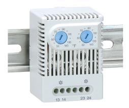
Stego thermostat, dual adjustable, N.O. (close on rise) 32 to 140 deg F, N.O. (close on rise) 32 to 140 deg F, 12.6 deg F switching differential, 35mm DIN rail mount, for electrical enclosure climate control.
