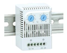
Stego thermostat, dual adjustable, N.O. (close on rise) 0 to 60 deg C, N.O. (close on rise) 0 to 60 deg C, 7K switching differential, 35mm DIN rail mount, for electrical enclosure climate control.
