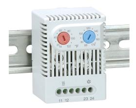
Stego thermostat, dual adjustable, N.C. (open on rise) 14 to 122 deg F, N.O. (close on rise) 68 to 176 deg F, 12.6 deg F switching differential, 35mm DIN rail mount, for electrical enclosure climate control.
