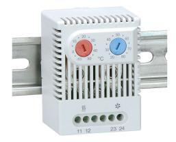
Stego thermostat, dual adjustable, N.C. (open on rise) -10 to 50 deg C, N.O. (close on rise) 20 to 80 deg C, 7K switching differential, 35mm DIN rail mount, for electrical enclosure climate control.
