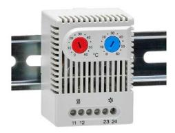
Stego thermostat, dual adjustable, N.C. (open on rise) 0 to 60 deg C, N.O. (close on rise) 0 to 60 deg C, 7K switching differential, 35mm DIN rail mount, for electrical climate control.
