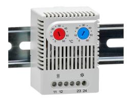
Stego thermostat, dual adjustable, N.C. (open on rise) 0 to 60 deg C, N.O. (close on rise) 0 to 60 deg C, 7K switching differential, 35mm DIN rail mount, for electrical enclosure climate control.
