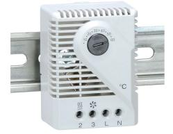
Stego mechanical thermostat, adjustable, 5 to 60 deg C, 5K switching differential, 120 VAC operating voltage, 35mm DIN rail mount, for electrical enclosure climate control.
