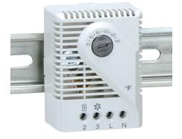
Stego mechanical thermostat, adjustable, 40 to 140 deg F, 9 deg F switching differential, 120 VAC operating voltage, 35mm DIN rail mount, for electrical enclosure climate control.
