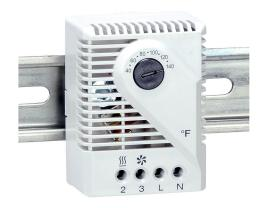
Stego mechanical thermostat, adjustable, 40 to 140 deg F, 9 deg F switching differential, 230 VAC operating voltage, 35mm DIN rail mount, for electrical enclosure climate control.
