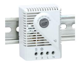
Stego mechanical thermostat, adjustable, 5 to 60 deg C, 5K switching differential, 230 VAC operating voltage, 35mm DIN rail mount, for electrical enclosure climate control.
