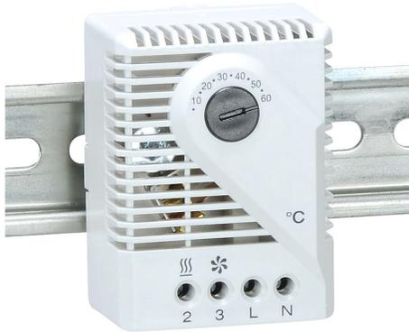
Stego mechanical thermostat, adjustable, 5 to 60 deg C, 5K switching differential, 230 VAC operating voltage, 35mm DIN rail mount, for electrical enclosure climate control.
