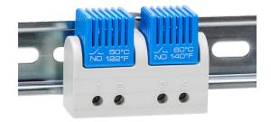
Stego thermostat, dual fixed, N.O. (close on rise) 122 deg F (50 deg C) switch-on, N.O. (close on rise) 140 deg F (60 deg C) switch-on, 18 deg F (10K) switching differential, 35mm DIN rail mount, for electrical enclosure climate control.
