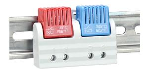
Stego thermostat, dual fixed, N.C. (open on rise) 41 deg F (5 deg C) switch-on, N.O. (close on rise) 95 deg F (35 deg C) switch-on, 18 deg F (10K) switching differential, 35mm DIN rail mount, for electrical enclosure climate control.
