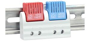
Stego thermostat, dual fixed, N.C. (open on rise) 41 deg F (5 deg C) switch-on, N.O. (close on rise) 95 deg F (35 deg C) switch-on, 18 deg F (10K) switching differential, 35mm DIN rail mount, for electrical enclosure climate control.
