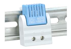
Stego thermostat, fixed, N.O. (close on rise) 122 deg F (50 deg C) switch-on, 12.6 deg F (7K) switching differential, 35mm DIN rail mount, for electrical enclosure climate control.
