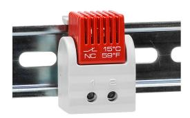
Stego thermostat, fixed, N.C. (open on rise) 41 deg F (5 deg C) switch-on, 18 deg F (10K) switching differential, 35mm DIN rail mount, for electrical enclosure climate control.
