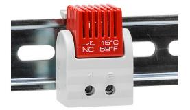
Stego thermostat, fixed, N.C. (open on rise) 41 deg F (5 deg C) switch-on, 18 deg F (10K) switching differential, 35mm DIN rail mount, for electrical enclosure climate control.
