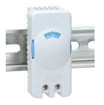
Stego thermostat, adjustable, N.O. (close on rise) 32 to 140 deg F, 7 deg F switching differential, 35mm DIN rail mount, for electrical enclosure climate control.
