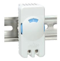
Stego thermostat, adjustable, N.O. (close on rise) 0 to 60 deg C, 4K switching differential, 35mm DIN rail mount, for electrical enclosure climate control.
