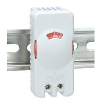
Stego thermostat, adjustable, N.C. (open on rise) 32 to 140 deg F, 7 deg F switching differential, 35mm DIN rail mount, for electrical enclosure climate control.
