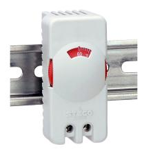
Stego thermostat, adjustable, N.C. (open on rise) 0 to 60 deg C, 4K switching differential, 35mm DIN rail mount, for electrical enclosure climate control.
