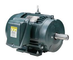
Toshiba SD premium efficiency AC induction motor, high-performance inverter duty and severe duty, 10hp, 3-phase, 230/460 VAC, 1800rpm, TEFC, NEMA 215T frame, cast iron, rigid base mount.
