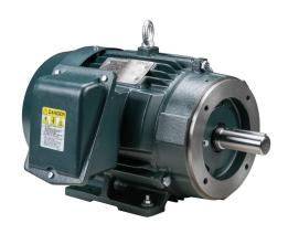
Toshiba SD premium efficiency AC induction motor, high-performance inverter duty and severe duty, 10hp, 3-phase, 230/460 VAC, 3600rpm, TEFC, NEMA 215TC frame, cast iron, C-face/rigid base mount.
