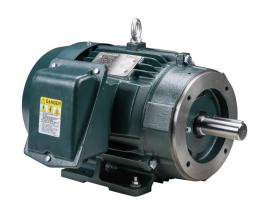
Toshiba SD premium efficiency AC induction motor, high-performance inverter duty and severe duty, 10hp, 3-phase, 230/460 VAC, 3600rpm, TEFC, 215TC frame, cast iron, C-face/rigid base mount.
