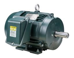
Toshiba SD premium efficiency AC induction motor, highperformance inverter duty and severe duty, 10hp, 3-phase, 230/460 VAC, 3600rpm, TEFC, NEMA 215T frame, cast iron, rigid base mount.
