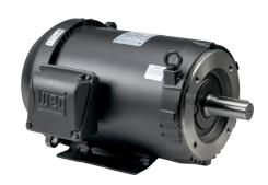
WEG Electric S premium efficiency AC induction motor, general purpose and inverter rated, 10hp, 3-phase, 208-230/460 VAC, 1800rpm, TEFC, NEMA 215TC frame, rolled steel, C-face/rigid base mount.
