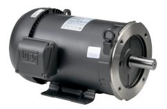
WEG Electric S premium efficiency AC induction motor, general purpose and inverter rated, 7-1/2hp, 3-phase, 208-230/460 VAC, 3600rpm, TEFC, NEMA 184TC frame, rolled steel, C-face/rigid base mount.
