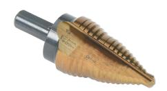
Viking step drill bit, 1/4in to 1-1/8in, size 1/4A, 16 steps, split point, high-speed steel (HSS), gold oxide finish, 3/8in diameter 3-flat shank, 3.0in (76mm) overall length.
