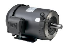
WEG Electric S premium efficiency AC induction motor, general purpose and inverter rated, 7-1/2hp, 3-phase, 208-230/460 VAC, 1800rpm, TEFC, NEMA 213TC frame, rolled steel, C-face/rigid base mount.
