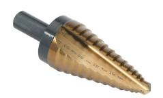
Viking step drill bit, 1/4in to 1in, size #2, 8 steps, split point, high-speed steel (HSS), gold oxide finish, 3/8in diameter 3-flat shank, 3.0in (76mm) overall length.
