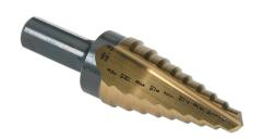
Viking step drill bit, 1/4in to 3/4in, size #3, 9 steps, split point, high-speed steel (HSS), gold oxide finish, 3/8in diameter 3-flat shank, 2.5in (64mm) overall length.
