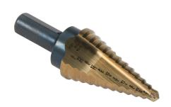
Viking step drill bit, 3/16in to 7/8in, size #8, 12 steps, split point, high-speed steel (HSS), gold oxide finish, 3/8in diameter 3-flat shank, 2.8in (71mm) overall length.
