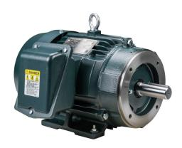
Toshiba SD premium efficiency AC induction motor, high-performance inverter duty and severe duty, 5hp, 3-phase, 230/460 VAC, 1200rpm, TEFC, 215TC frame, cast iron, C-face/rigid base mount.
