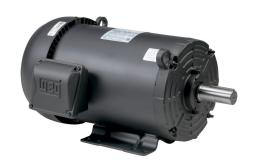
WEG Electric S premium efficiency AC induction motor, general purpose and inverter rated, 5hp, 3-phase, 208-230/460 VAC, 3600rpm, TEFC, 184T frame, rolled steel, rigid base mount.
