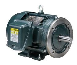
Toshiba SD premium efficiency AC induction motor, high-performance inverter duty and severe duty, 5hp, 3-phase, 230/460 VAC, 3600rpm, TEFC, NEMA 184TC frame, cast iron, C-face/rigid base mount.
