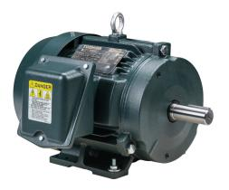
Toshiba SD premium efficiency AC induction motor, highperformance inverter duty and severe duty, 5hp, 3-phase, 230/460 VAC, 3600rpm, TEFC, NEMA 184T frame, cast iron, rigid base mount.
