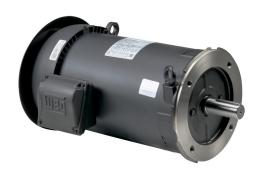
WEG Electric S premium efficiency AC induction motor, general purpose and inverter rated, 5hp, 3-phase, 208-230/460 VAC, 1800rpm, TEFC, 184TC frame, rolled steel, C-face mount. Drip cover included.
