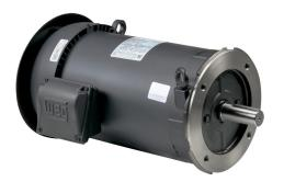
WEG Electric S premium efficiency AC induction motor, general purpose and inverter rated, 5hp, 3-phase, 208-230/460 VAC, 1800rpm, TEFC, NEMA 184TC frame, rolled steel, C-face mount. Drip cover included.
